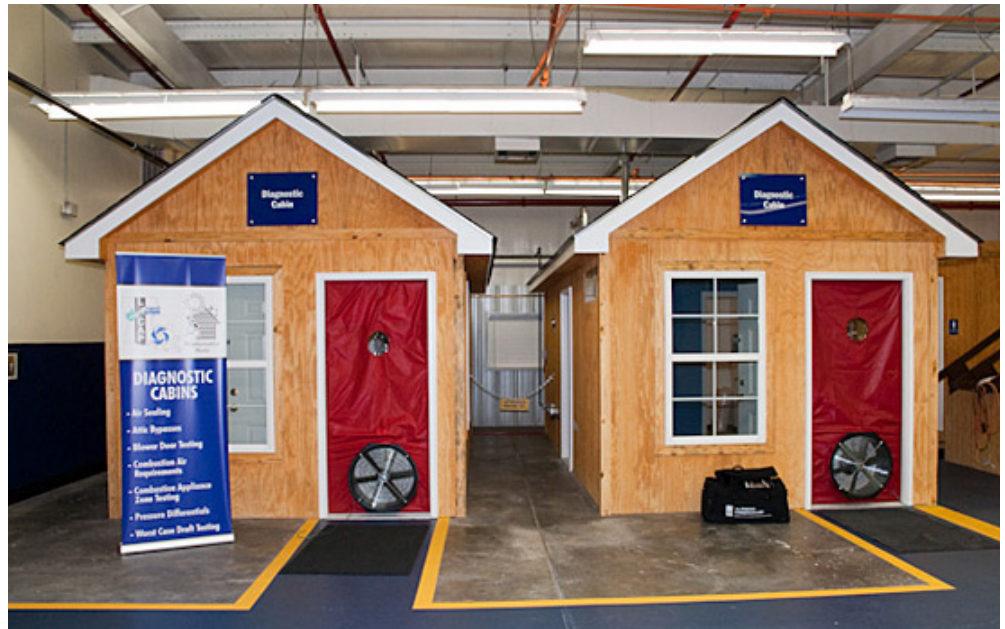
The LACAP training center provides three diagnostic cabins for students to use for the “house as a system” training, which includes blower door tests and live combustion appliances.
